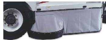
Sealed dust skirts control thick dust and thick powder
