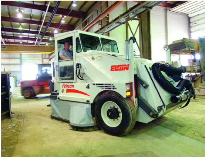
Dry operation allows powderous material sweeping
