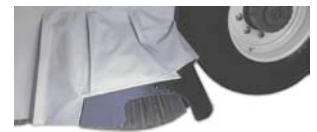
Optional: Cut out dust skirts allow clean curb sweeping
