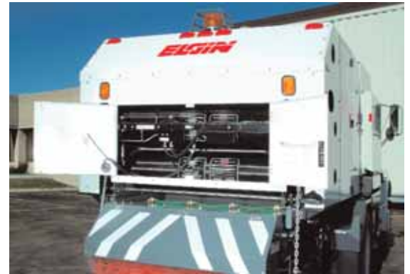
Easy fuel system service at rear of sweeper
